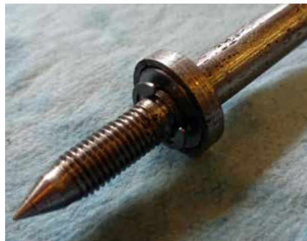
Valve open ----- Valve closed Needle portion of valve can be seen at the base of the rod
