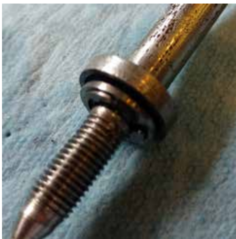
Valve open ----- Valve closed Needle portion of valve can be seen at the base of the rod
