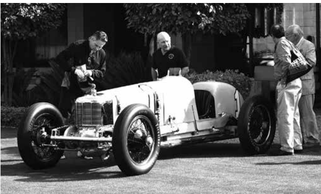
1925 Miller Junior Eight – The first front-wheel-drive car to race in the Indianapolis 500. The supercharged Miller was driven to a second-place finish by Dave Lewis in 1925 at an average speed just over 100 miles per hour.
